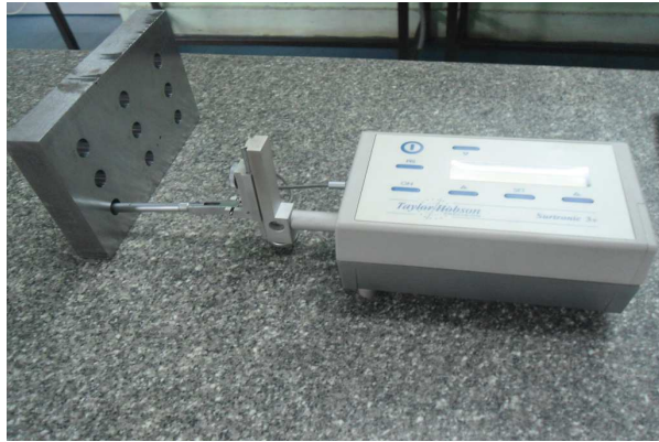
Figure 4: A Photograph of the Surface Roughness Tester
