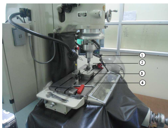
Figure 1: Experimental Set-up for Jig Grinding (1. Spindle, 2.Tool 3.Workpiece, 4.Work Table)
